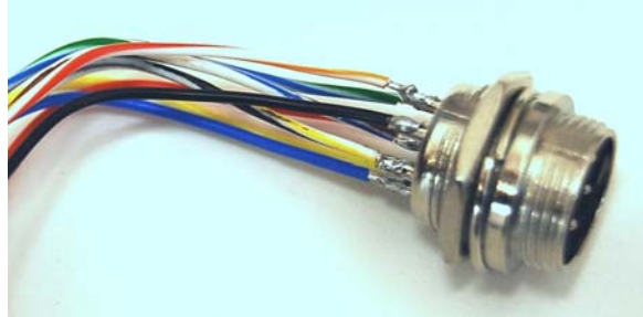
Different wire colors make it easy to keep track of microphone jack pin numbers.
