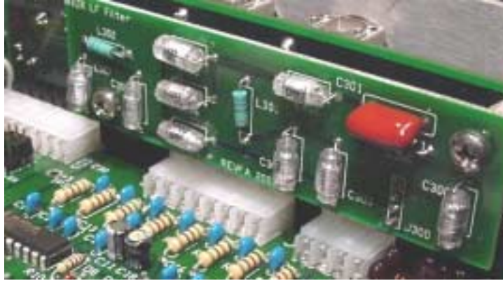
LF/AM Filter Mounted on Rear Panel
