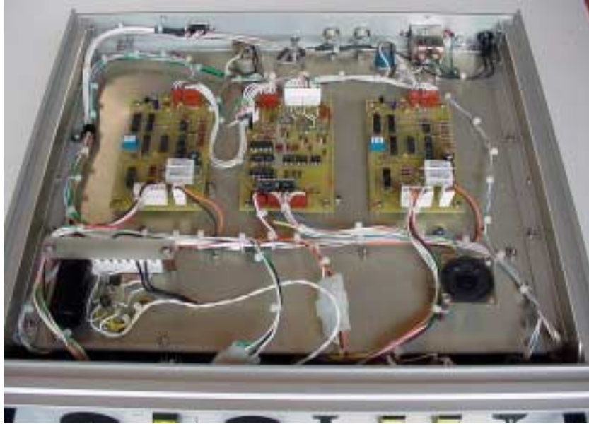
Figure 5—The 3"x5" controller circuit board, center, is shown flanked by two stepper motor driver boards in this underchassis view. A 5V -1A power supply is visible on the front left of the chassis, and a small "beep" speaker on the front right. The wiring harnesses use Teflon insulated wire secured with nylon fasteners. A combination 120 VAC receptacle/power line filter is visible at the right rear.
