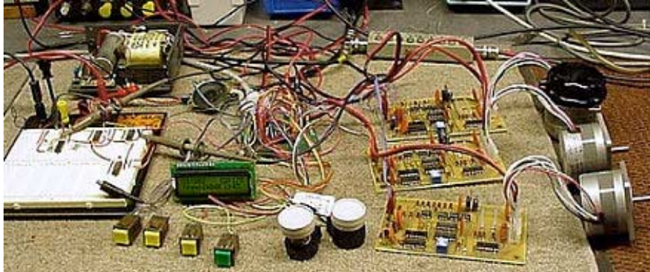
Figure 8—The EZ-Tuner started life as a snarl of wires and breadboarded components. The BS2sx microcontroller is buried in the rat's nest in the center.
