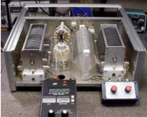
Figure 6— Setting the inductor taps is easy when using an MFJ-259B analyzer and AI1H's geometric resistance box, to simulate loads up to 32:1 VSWR. The tap-setting method described in the text uses only a 50 \Omega load.
