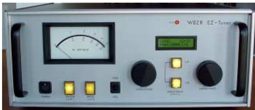
Figure 1—The EZ-Tuner's 16"x7" brushed aluminum front panel is dominated by the large r.f. wattmeter. Press-on letters from an art supply store were used to label the controls. After lettering was completed, two coats of satin finish clear plastic spray sealed the panel.
