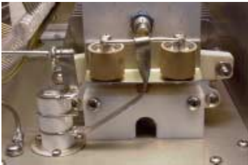
Figure 4—Two 50 pF 5000V capacitors are fixed to the back plate of the output variable capacitor with a small bracket and are switched into the circuit by a Jennings RF3A vacuum relay. Teflon blocks insulate the variable capacitors from the chassis.
