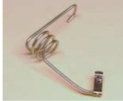
Figure 7— If the parts layout won't allow placing a tap just where it's needed, a smidgen of inductance can be added to the tap itself.
