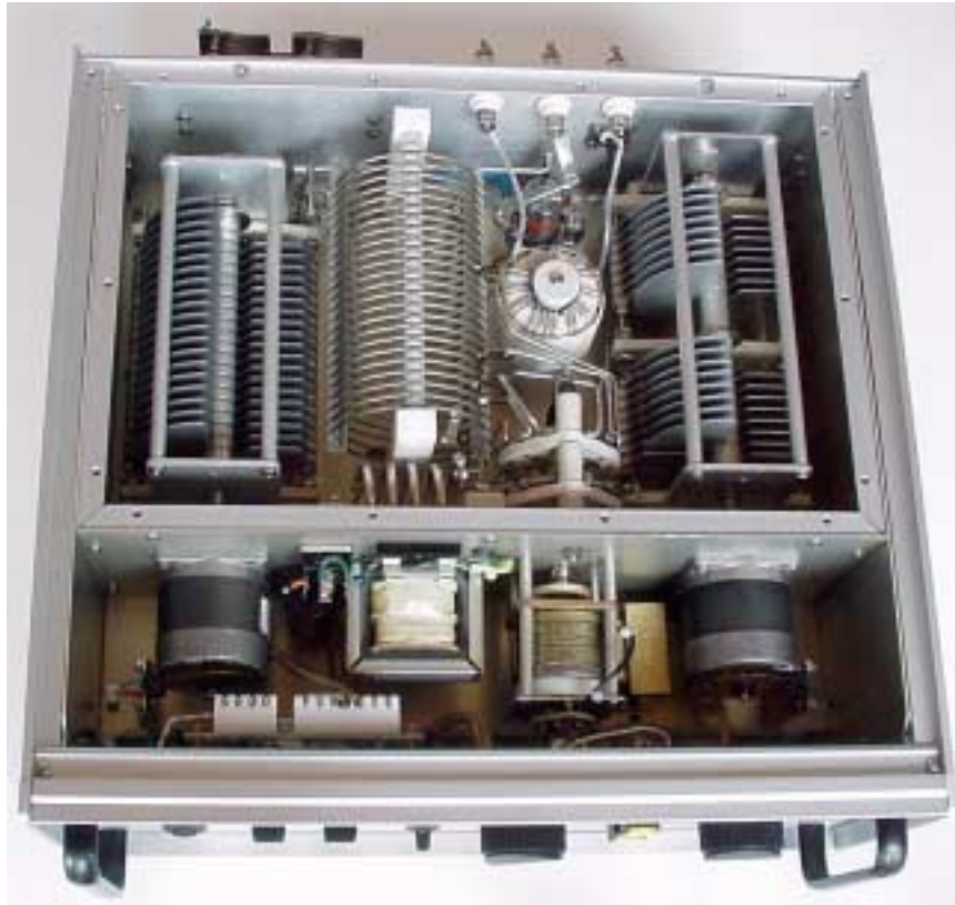
Figure 1—Stepper motor and a rotary solenoid shafts extend into the sealed r.f. subenclosure to operate the T-network capacitors and inductor switch. The 4:1 balun is visible behind the inductor switch.
