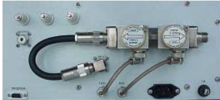
Figure 6 —The serial programming port is visible on the bottom left of the rear panel of the EZ-Tuner. A Bird dual line section measures forward and reflected r.f. power.
