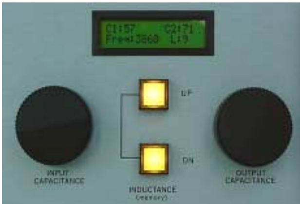
Figure 7 —In the manual mode, knob-turned optical encoders adjust the variable capacitors, and pushbuttons rotate the inductor switch. In the automatic mode, the pushbuttons ramp the EZ-Tuner through its 134 memories.
