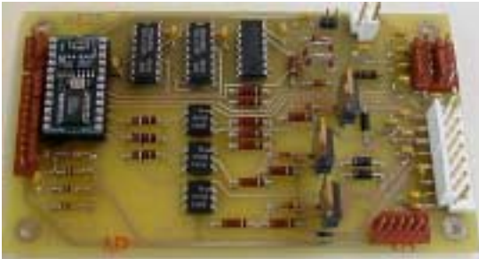
Figure 4 —The BASIC Stamp BS2sx is in the left rear of the 3x5 inch printed circuit controller board.
