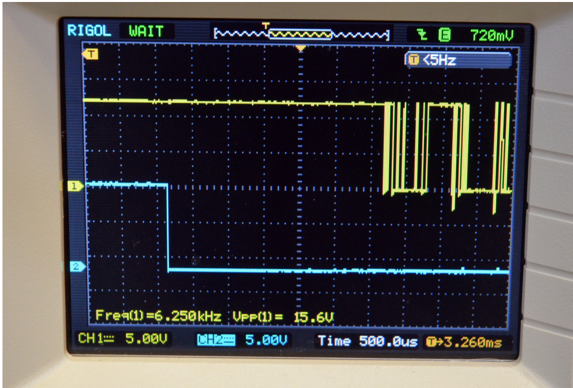
Figure 2: Timing comparison of a Jennings RJ1a (bottom curve) and a Gigavac G41c (top curve) vacuum relay. The RJ1a contact closes in 1.2 mS and shows no contact bounce, making it well suited for QSK operation. By contrast, the G41c contact closes in about 5.9 mS and shows appreciable contact bounce.
