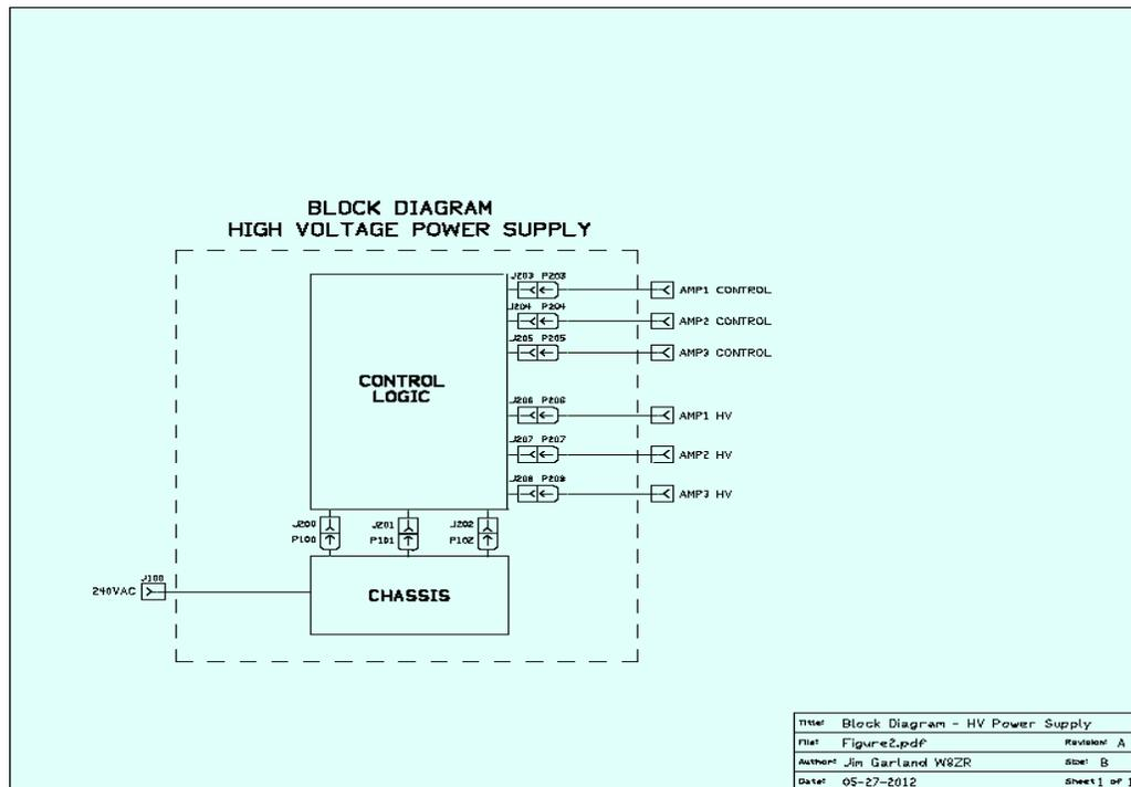
**Figure 2: The heart of the power supply is a control logic circuit that arbitrates among three connected RF decks, allowing fully automatic operation.**
