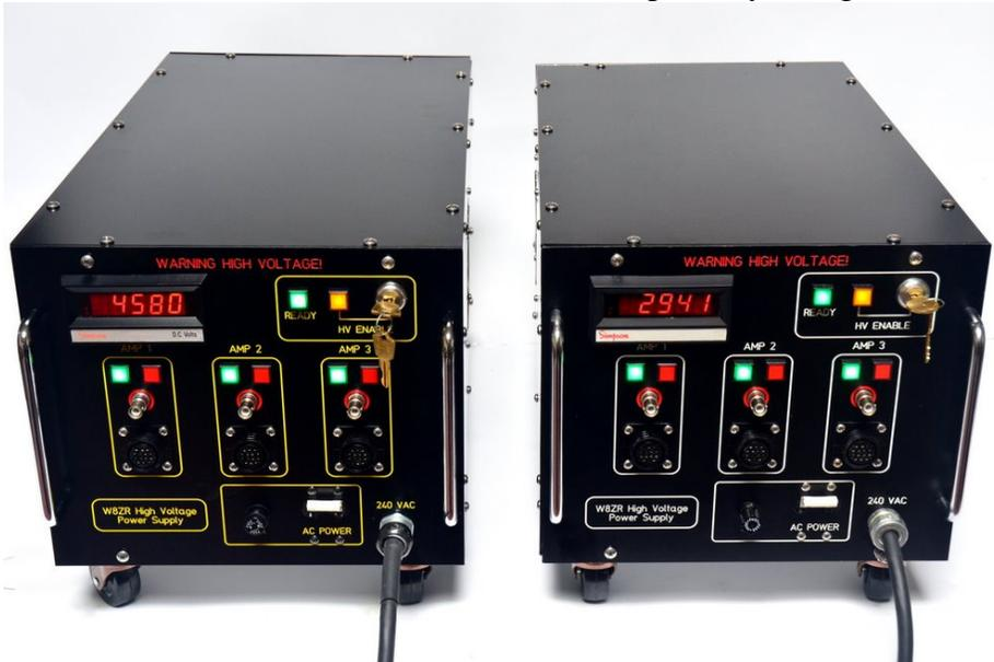
**Figure 1: The high voltage power supplies, identical except for different voltage ranges, rest on the floor behind an operating table and independently power up to three legal-limit RF power amplifiers.**
