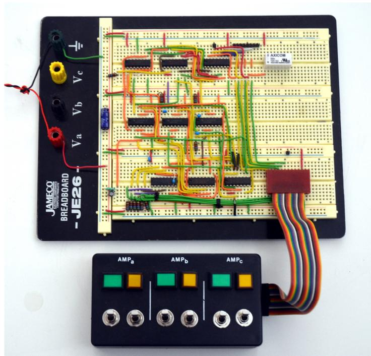
Figure 11: The logic and control circuitry was tested and debugged with this breadboard mockup, before laying out the printed circuit board.
