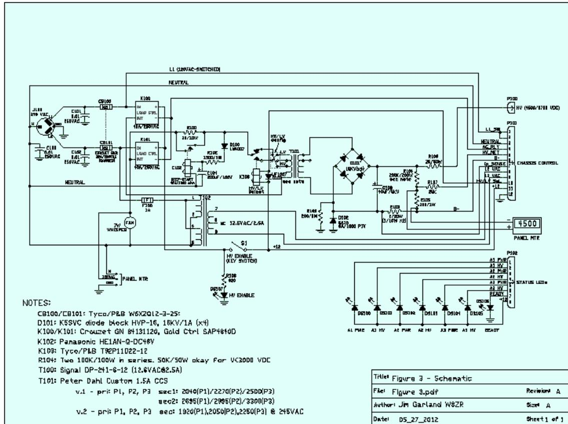
**Figure 3: Schematic diagram of the high voltage circuits.**The power supply uses a capacitor input filter with a large oil-filled capacitor filtering the rectified output from the full-wave bridge rectifier. An “HV Enable” key-operated safety switch disables the plate transformer by deactivating the solid state power relays.
