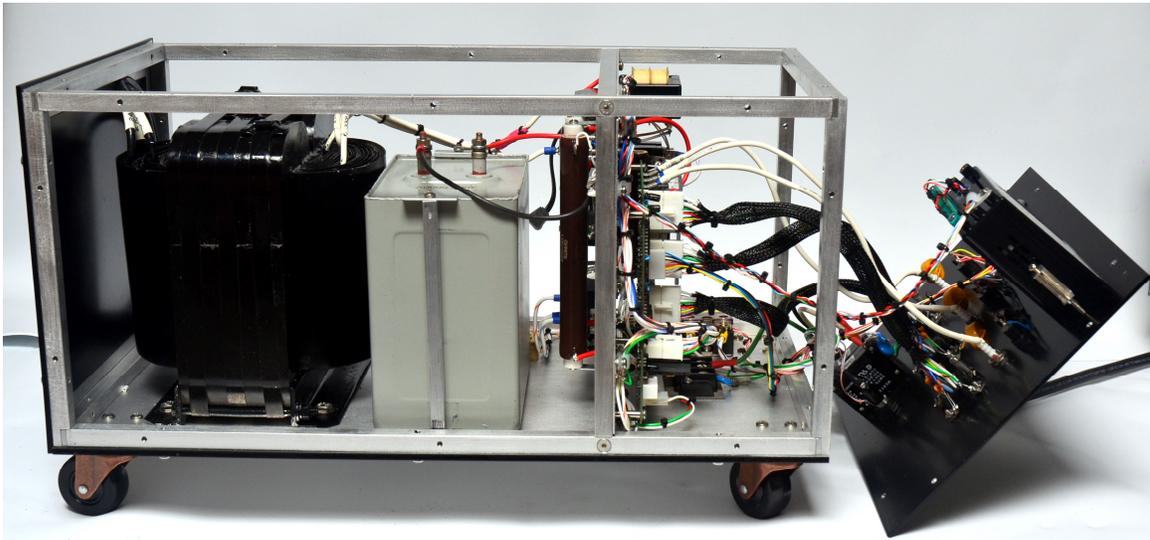
**Figure 6:** The front panel detaches and tilts forward for servicing and access to the logic and control circuitry.
